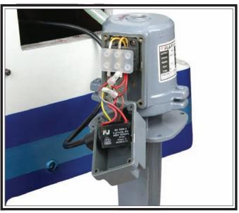
Figure 70. Coolant pump motor wiring.
